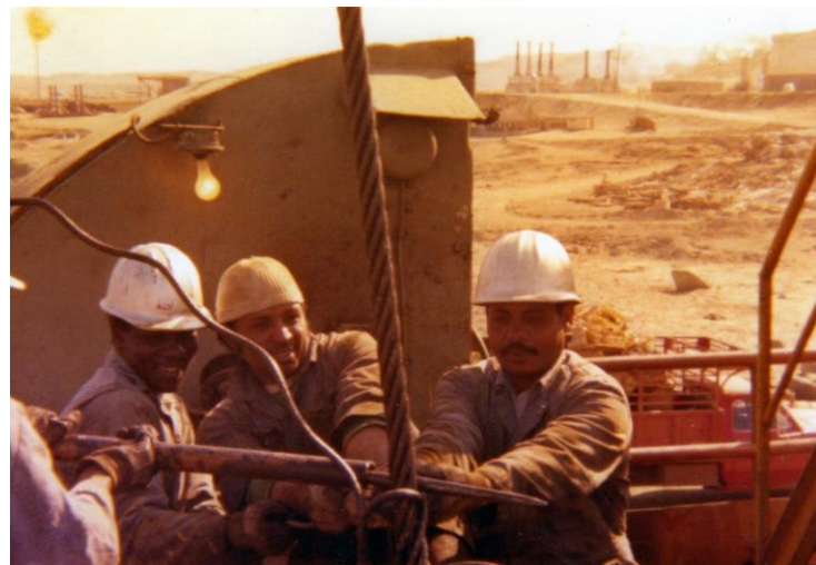
Teaching members of the crew how to splice a 3inch wire bridle for towing,
