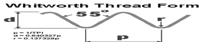
The above diagram shows the characteristics of the Whitworth tread as developed by Sir Joseph Whitworth. The Whitworth tread was also known as British Standard Whitworth or BSW for short, and due to its' popularity with British manufacturers it was used on a large number of machinery which was exported to the four corners of the globe, thus making its' mark as a world leader of its' time.
